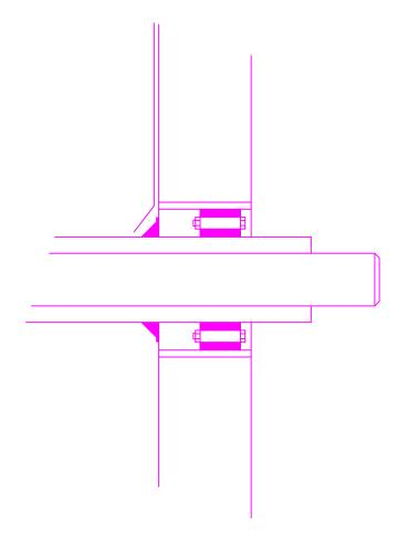
SLEEVE AND SEAL ASSEMBLY DETAIL (WITH WATERPROOFING MEMBRANE) SCALE: NO SCALE
